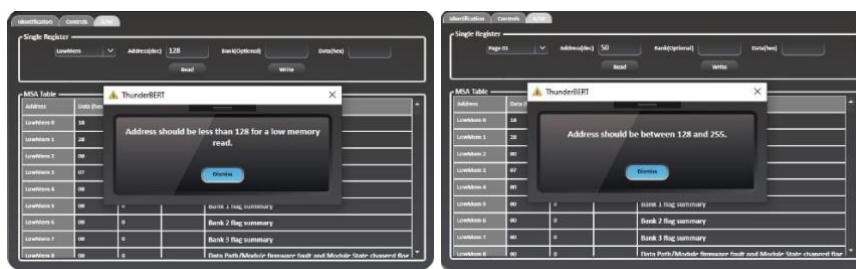
Figure 59: Warning pop-up messages when the address access conditions were not adhered to
