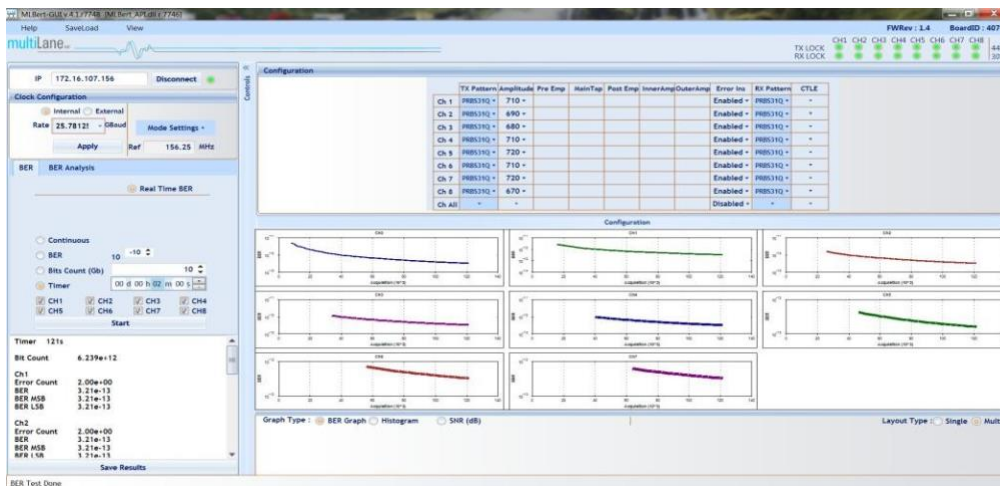
Figure 41: BER measurement with 1 error inserted at the MSB and 1 error at the LSB
