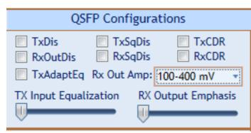
Figure 21 QSFP configuration bits
