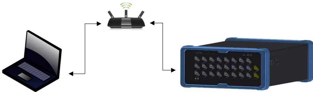
Figure 3: ML4035 connected to PC via Ethernet
