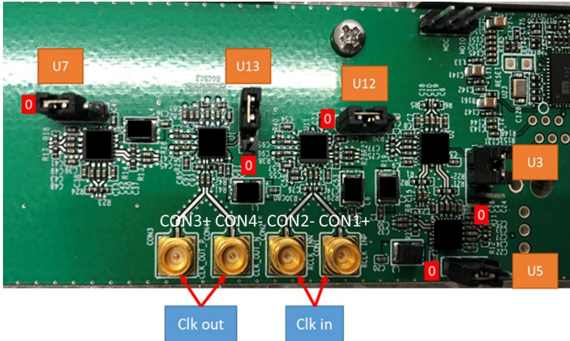
Figure 15: AT93000 Backplane - Clock routing jumpers
