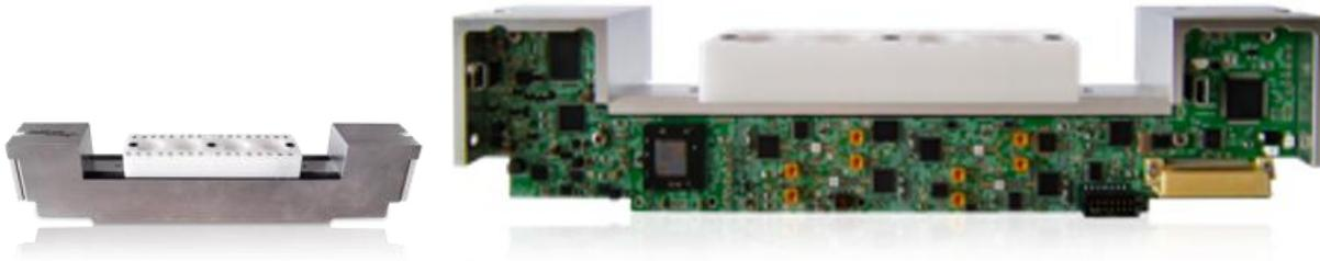
Figure 4: Instrument Cassette with protective cover removed
