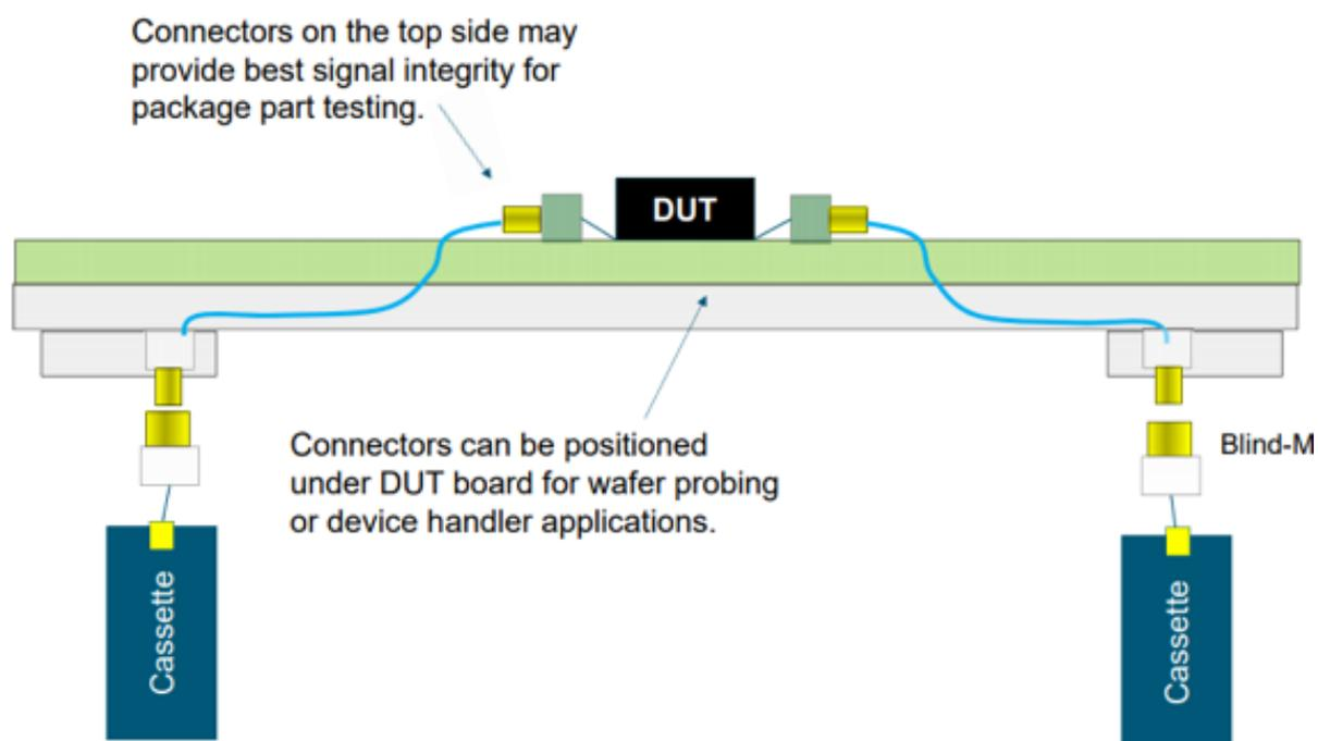
Figure 6: Signal path of the ATE system
