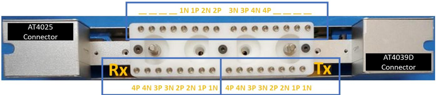
Figure 9: Same AT4039D + AT4025 cassette rotated 180 degrees
