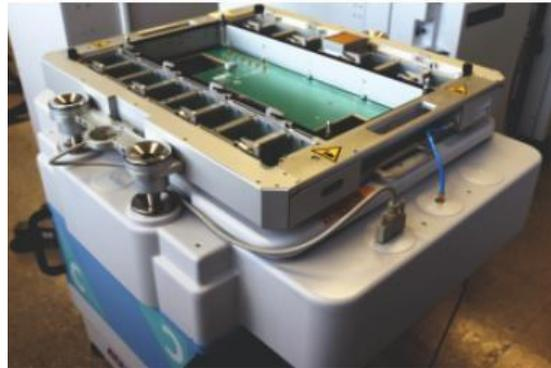
Figure 1: V93k CTH testhead with Multilane AT93000 system attached on top
