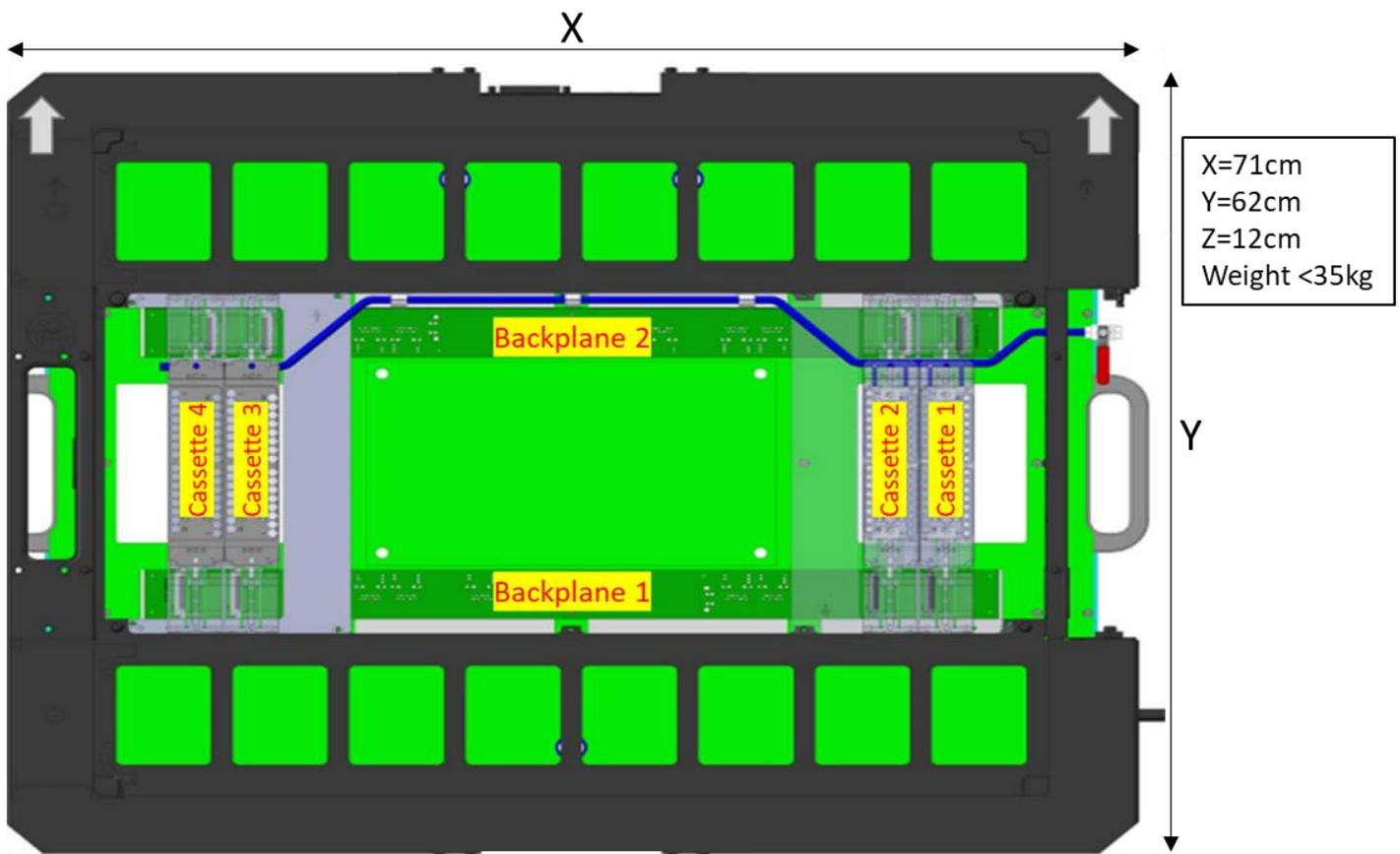
Figure 7: (Top View) AT93000 Backplane and Cassette numbering
