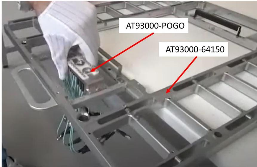
Figure 30: AT93000-POGO being installed onto loadboard
