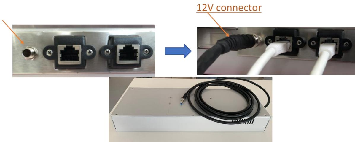
Figure 25: AT93000 Power Supply
