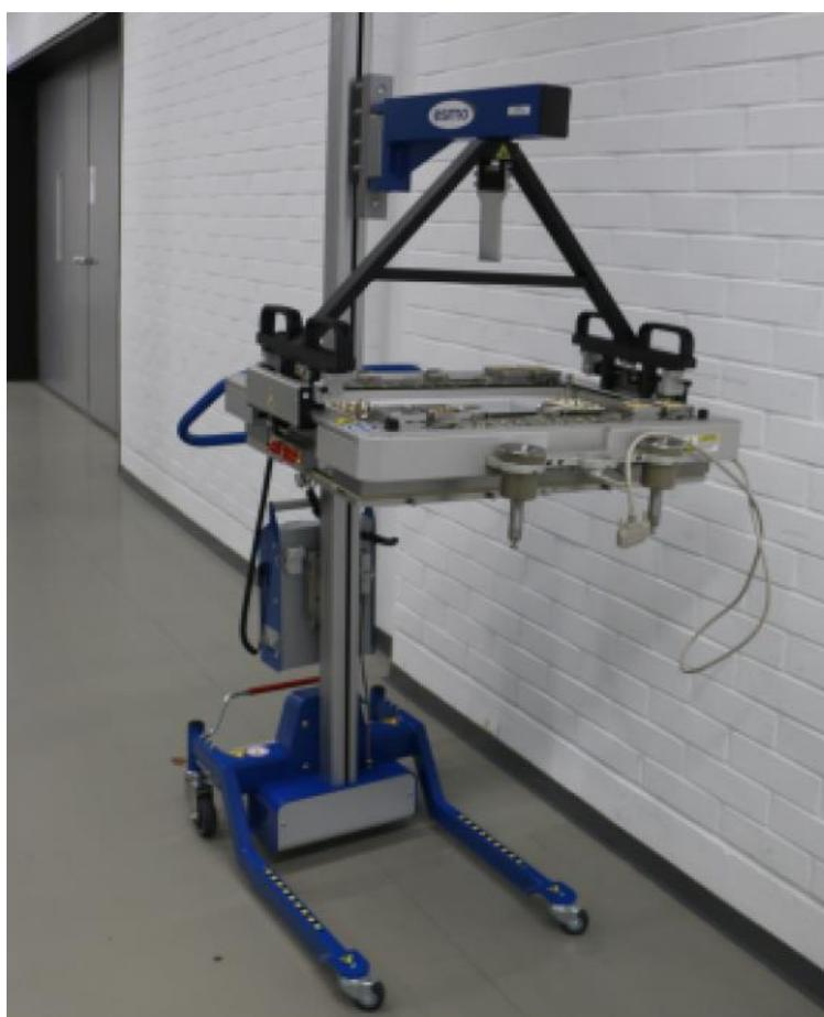
Figure 26: AT93000 twinning lift described in the Advantest documentation
