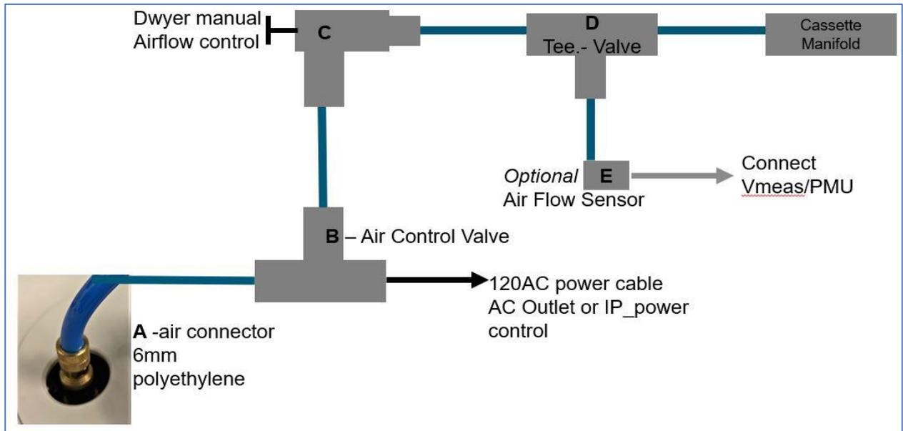
Figure 22: Schematic view of cooling air path
