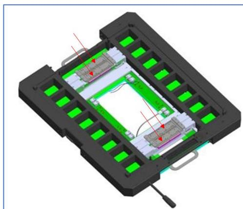
Figure 3: ML AT93000 system with red arrows pointing to the 4 Multilane cassettes
