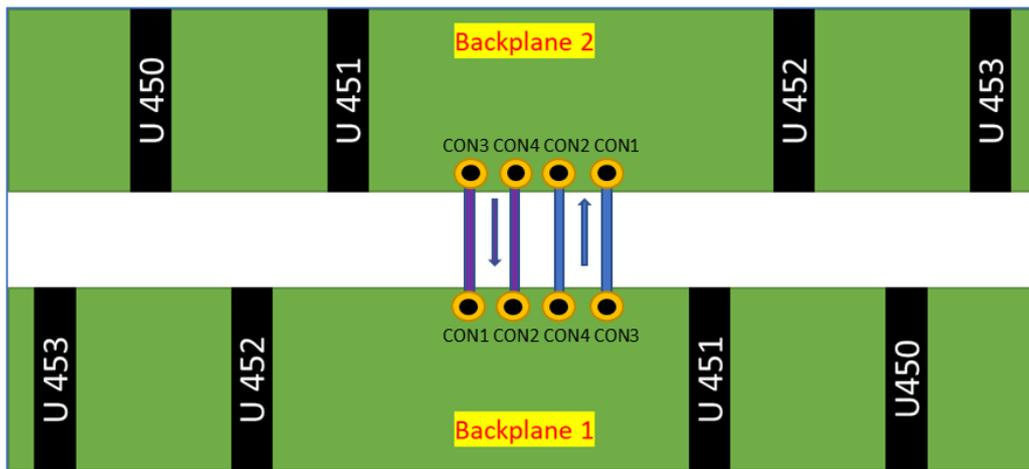
Figure 16: AT93000 Backplane - Connectors Numbers
