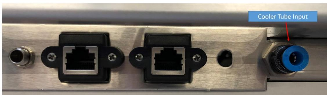
Figure 20: AT93000 Cooler Tube Input
