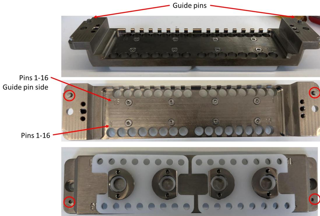
Figure 32: AT93000-POGO with guide pins
